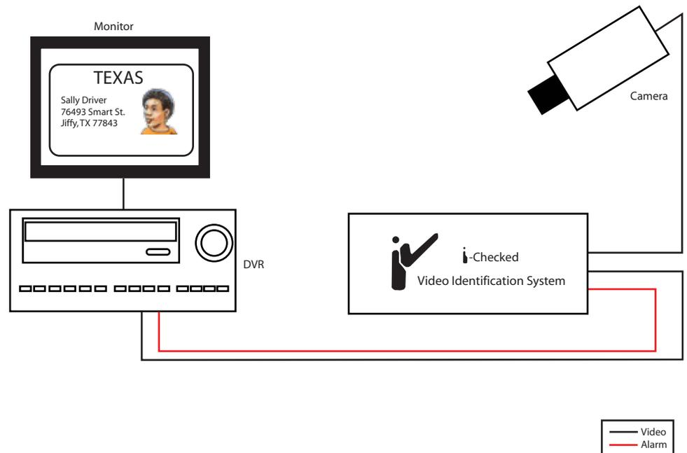
The i-Checked is easy to install in a new or existing CCTV system. The standard Alarm output links to DVR to provide a record of each ID checked in the DVR's event list.
