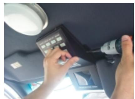
View of control console being mounted with wires already attached to connections
