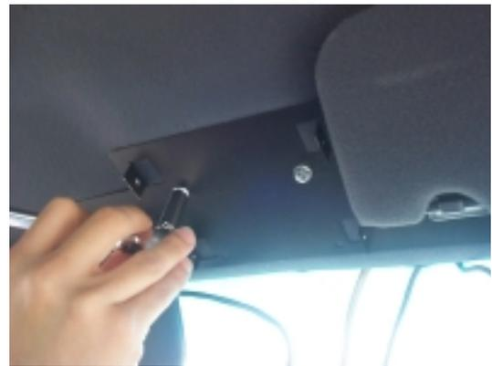
Attaching the Control head mounting plate between the sun visors.
